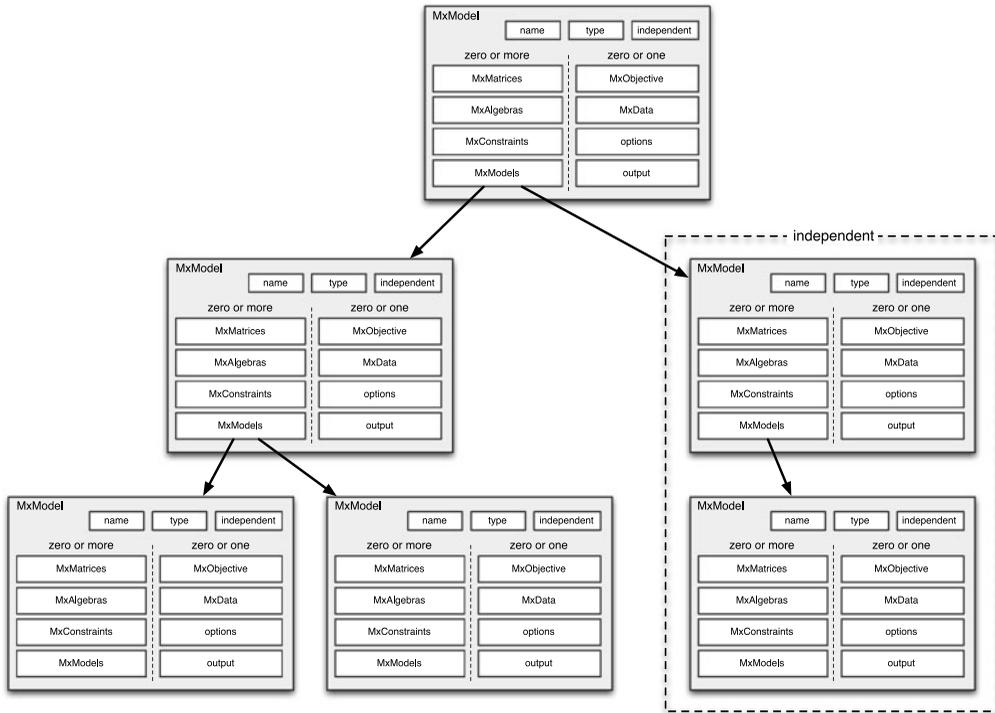
FIGURE 3. MxModels can contain lists of submodels.
