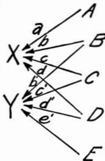
FIG. 2.—Diagram showing relations between two variables, X and Y , whose values are determined in part by common causes, B, C, and D , which are independent of each other.
